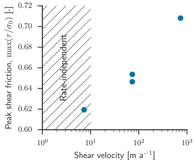
**Figure 6.** Peak frictional strength before the critical state of the low-permeability granular bed ( $k_c = 3.5 \times 10^{-15} \text{ m}^2$ ) at different shear velocities. The frictional strength is constant and rate independent at velocities lower than  $10^1 \text{ m a}^{-1}$  as pore-pressure diffusion rates far exceed rates in volumetric change.
