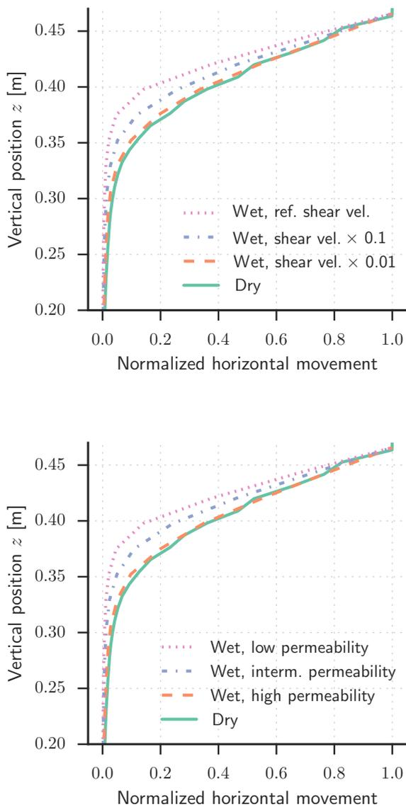
**Figure 8.** Horizontal particle displacement with depth (shear strain profiles) for the dry and fluid-saturated shear experiments. Top: displacement profiles from experiments with different shear velocities. Bottom: displacement profiles from experiments with different permeabilities.
