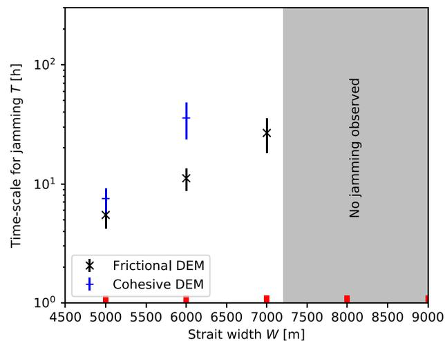
**Figure 8.** Jamming behavior with increasing width of the strait (Figure 5) for Coulomb frictional ( $\mu = 0.3$  and  $\sigma_c = 0$  kPa) and cohesive runs ( $\mu = 0$  and  $\sigma_c = 200$  kPa). The frictional model does not show jamming above  $W = 7,000$  m, and the cohesive model does not show jamming above  $W = 6,000$  m. Red ticks denote tested values. DEM = discrete element method.
