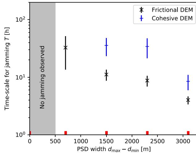
**Figure 9.** Jamming behavior with increasing width of the particle size distribution for Coulomb frictional ( $\mu = 0.3$  and  $\sigma_c = 0$  kPa) and cohesive runs ( $\mu = 0$  and  $\sigma_c = 200$  kPa). Red ticks denote tested values. DEM = discrete element method.
