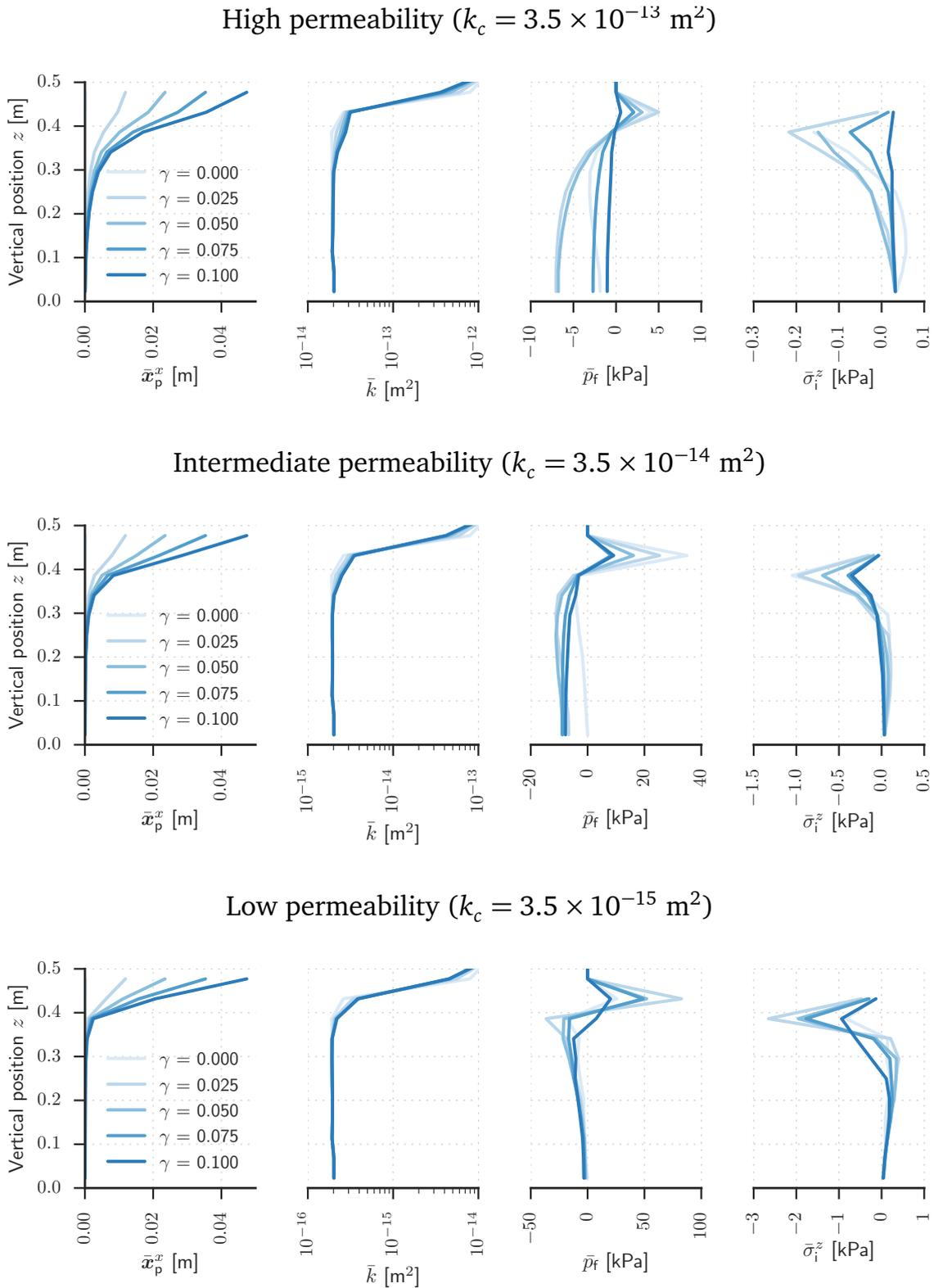
**Figure 10.** Horizontally averaged fluid and particle behavior with progressive shear strain. (left) Vertical particle displacement, (center left) mean permeability, (center right) mean fluid pressure, and (right) vertical component of the mean fluid stress, calculated as  $f_1^i/A^i$ , where  $f_1^i$  is the fluid pressure force on particle  $i$  from Eq. (12) and  $A^i$  is its surface area. Note that the limits of the horizontal axes differ between the experiments.
