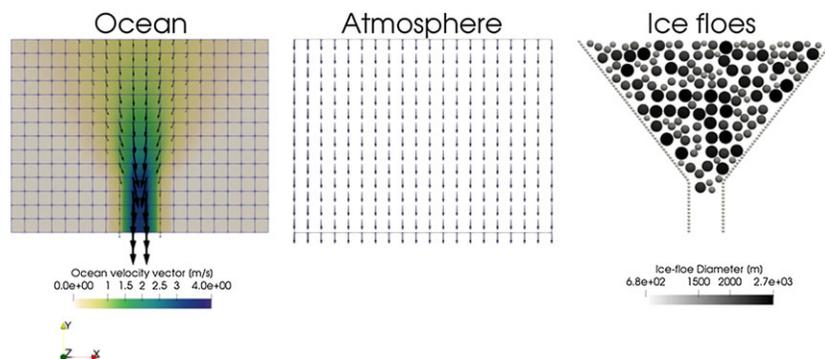
**Figure 2.** Simulation setup for the idealized strait experiments. Ocean velocities vary from 0 to 4 m/s relative to the bounding geometry, while the atmosphere velocity field is a uniform value of 30 m/s.
