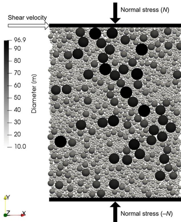
**Figure 1.** Simulation setup for the simple shear experiments. The upper and lower walls exert a prescribed normal stress to the granular assemblage, and a constant velocity along  $x$  is enforced for the uppermost ice floes. Left and right ( $-x$  and  $+x$ ) boundaries are periodic.
