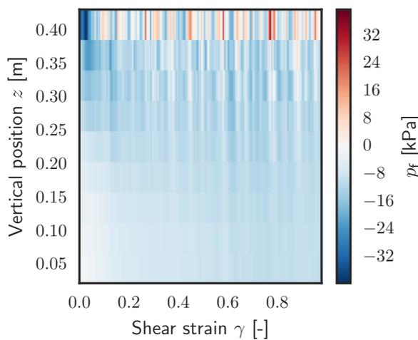
**Figure 11.** Temporal evolution ( $x$  axis) of horizontally averaged fluid pressures ( $y$  axis). The permeable material (top) is able to quickly respond to internal volumetric changes, which are short-lived and of small magnitude. The low-permeability material (bottom) is dominated by large pressure reductions and relatively slow relaxation.
