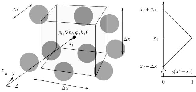
**Figure 2.** Left: a cell in the fluid grid. The node for pressure ( $p_f$ ), the gradient of fluid pressure ( $\nabla p_f$ ), porosity ( $\phi$ ), permeability ( $k$ ), and average grain velocity ( $\bar{v}$ ) are calculated at the cell center. Right: the weight function (Eq. 6) at various distances.
