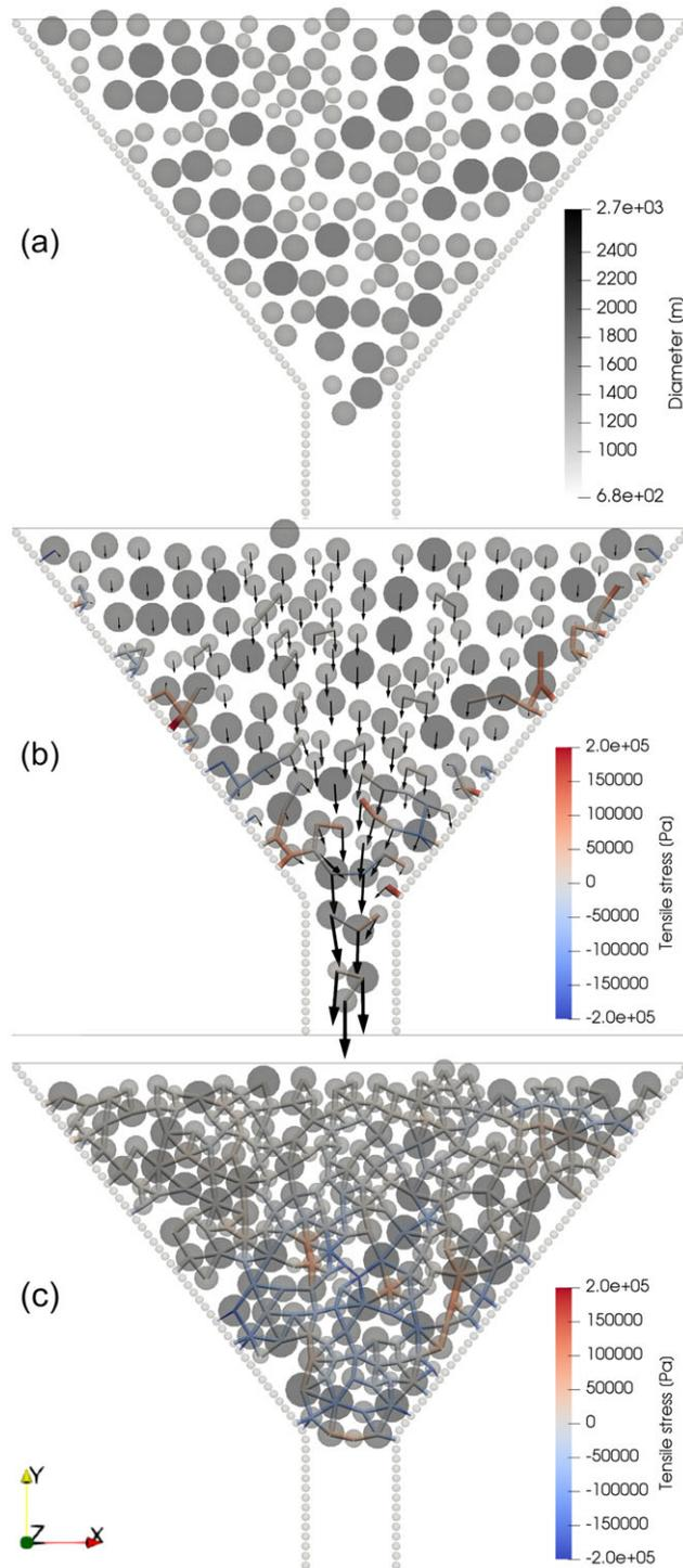
**Figure 5.** Example visualization of the granular system for the *idealized strait* runs, here the initial state (a), during flow (b), and in a jammed state (c). Black arrows denote the linear velocity of the ice floes, and colored bars indicate compressive or tensile granular interactions. The above visualizations are for run 1 out of 10 with  $\mu = 0$  and  $\sigma_c = 400$  kPa.
