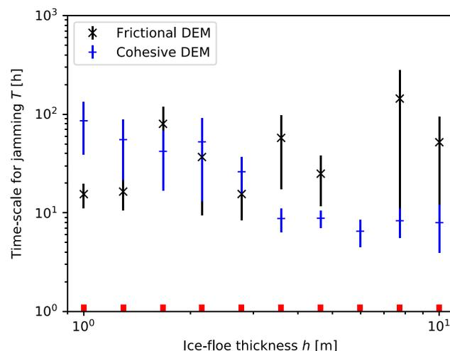
**Figure 10.** Jamming behavior with uniformly increasing thickness of the ice floes for Coulomb frictional ( $\mu = 0.3$  and  $\sigma_c = 0$  kPa) and cohesive runs ( $\mu = 0$  and  $\sigma_c = 200$  kPa). Red ticks denote tested values. DEM = discrete element method.
