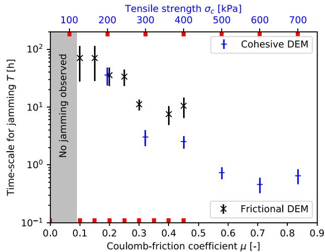
**Figure 7.** The influence of the Coulomb frictional coefficient  $\mu$  (equation (10)) and the tensile strength  $\sigma_c$  (equation (11)) on the characteristic time for jamming  $T$  (equation (1)) through a strait of width  $W = 6,000$  m. A statistically significant fit could not be achieved from the Coulomb frictional ensemble with  $\mu = 0.35$ . Red ticks denote tested values. DEM = discrete element method.
